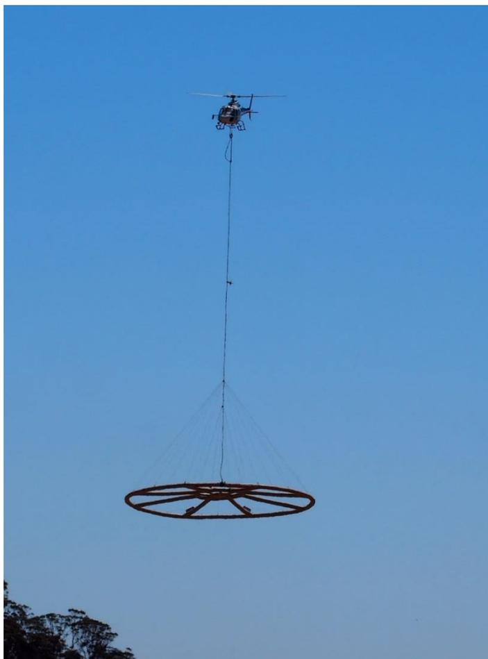
Figure 1: NRG helicopter undertaking AEM survey over E70/4688
