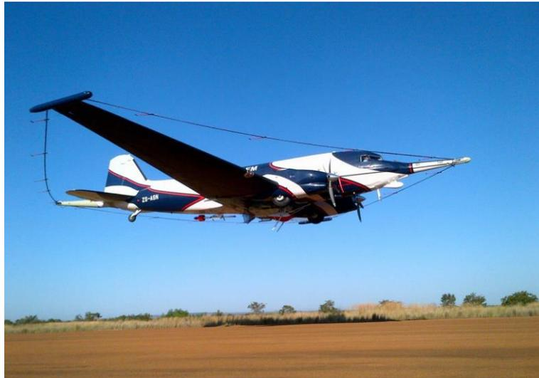
**Figure 2. Spectrem Airborne EM aircraft**
